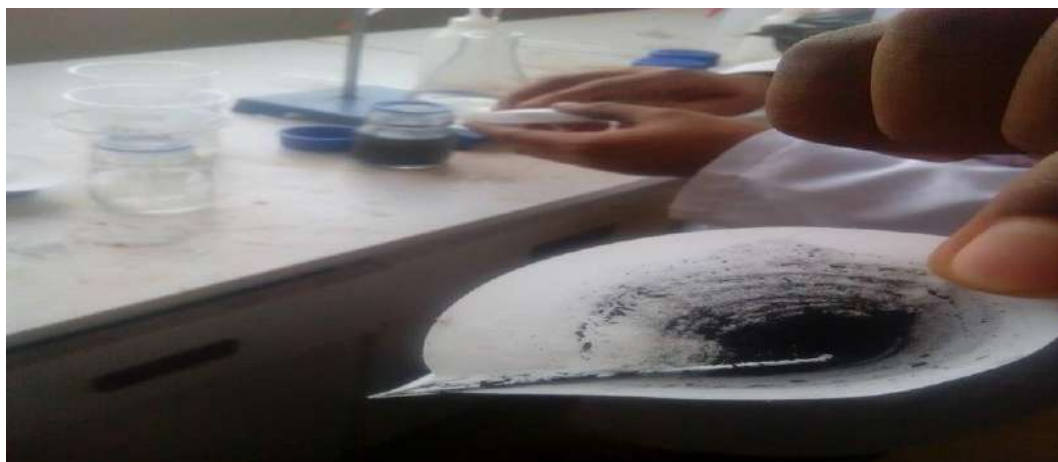
Fig 3: Remaining part of the adsorbent with Cu (II) ions being adsorbed
